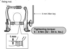
Pass the inner cable through the inner cable lead, and after setting so that the total of the clearances between the left and right shoes and the rim is 2 mm, tighten the cable fixing bolt.
