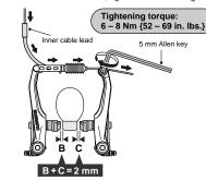
5. Adjust the bala with the spring tension adjustment screws.
