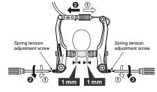
**6.** Depress the brake lever about 10 times as far as the grip and check that everything is operating correctly and that the shoe clearance is correct before using the brakes.
