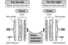
**3.** Insertion of shoe fixing pin is very critical to keep shoe properly fixed in place.
