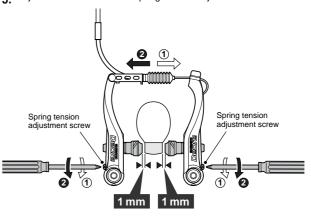
6. Depress the brake lever about 10 times as far as the grip and check that everything is operating correctly and that the shoe clearance is correct before using the brakes.
